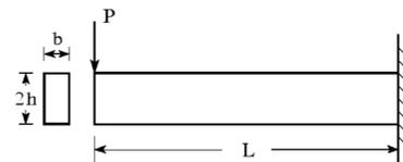
Calculate the expressions for **Stress, Strain, and Displacement** of the above loading situation, using both the Elasticity and Mechanics of Materials analysis methods.
