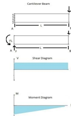
Now that we have the reaction forces for this particular case we can use them to solve the bending stress induced and in-turn the strain in the system. The bending stress in the beam can be seen in the diagram below. The magnitude of the stress is governed by the following equation:
